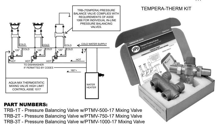
Precision Plumbing provides the first High Limit Thermostatic/Pressure Balance Control Package for two handle mixing valves.
